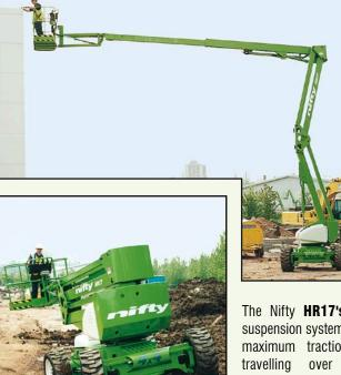
The Nifty **HR17's** unique suspension system ensures maximum traction when travelling over uneven ground and the 1.8m wide platform allows the operator ample space for tools.
